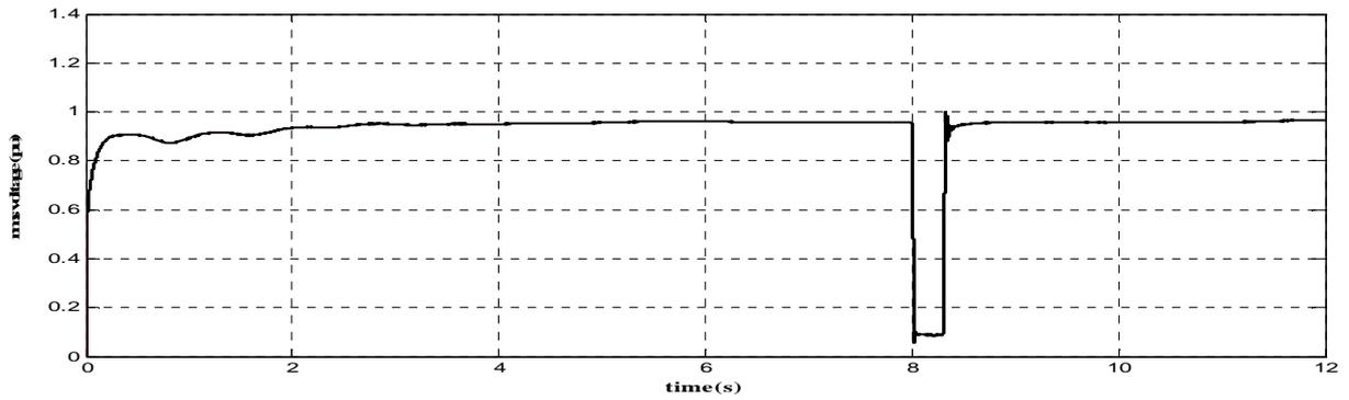
Fig.3 Rms\_voltage of the grid at the point of common coupling pre- and after fault clearance
