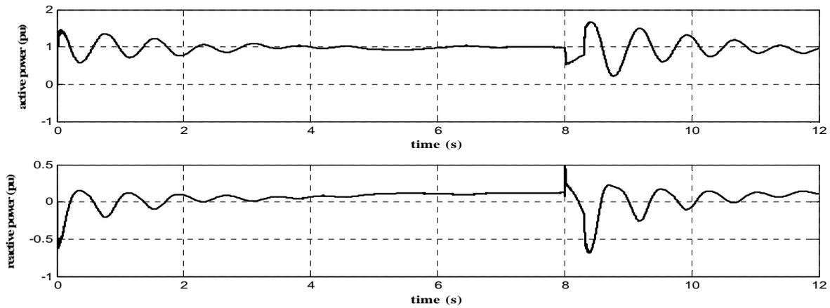
Fig.9 active and reactive power of the synchronous generator pre- and after fault clearance
