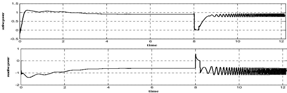
Fig.21 active and reactive power of the squirrel-cage induction generator pre- and after fault clearance
