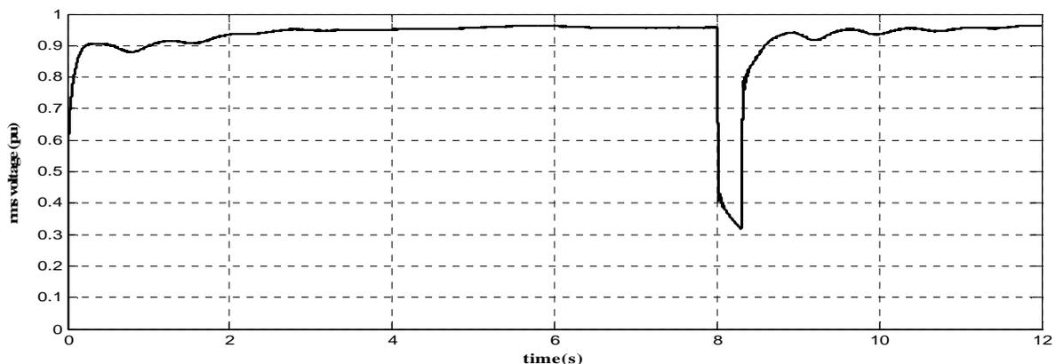
Fig. 8 Rmss\_voltage of the power system at the point of common coupling pre- and after fault clearance
