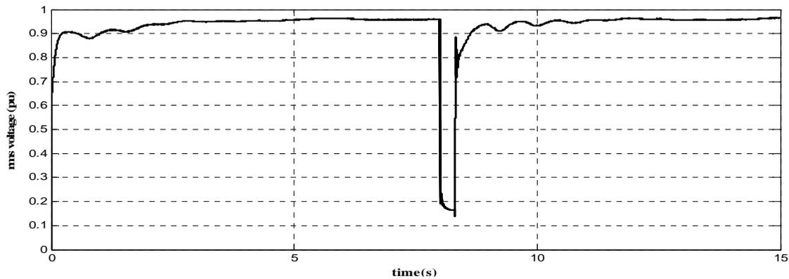
Fig.13 Rms\_voltage of the power system and at the point of common coupling pre- and after fault clearance
