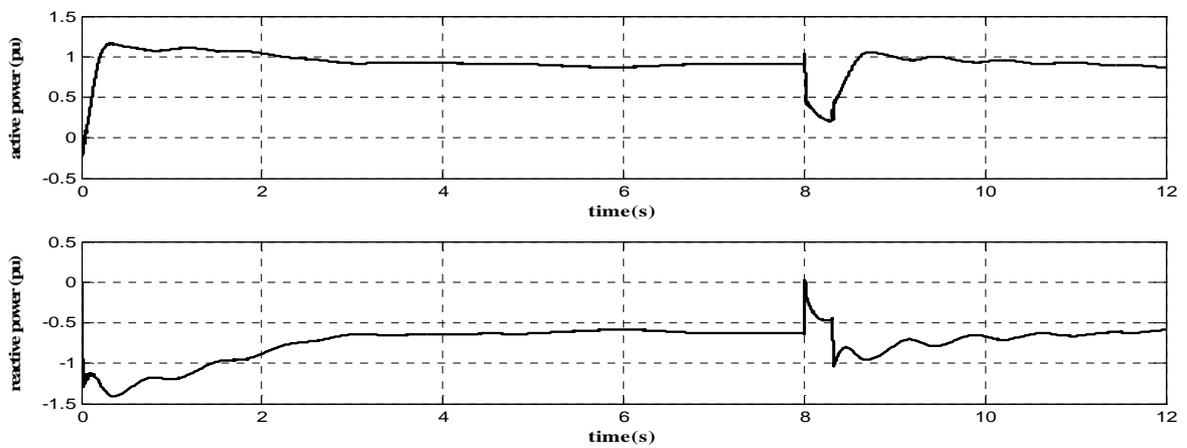
Fig.10 active and reactive power of the squirrel- cage induction generator pre- and after fault clearance
