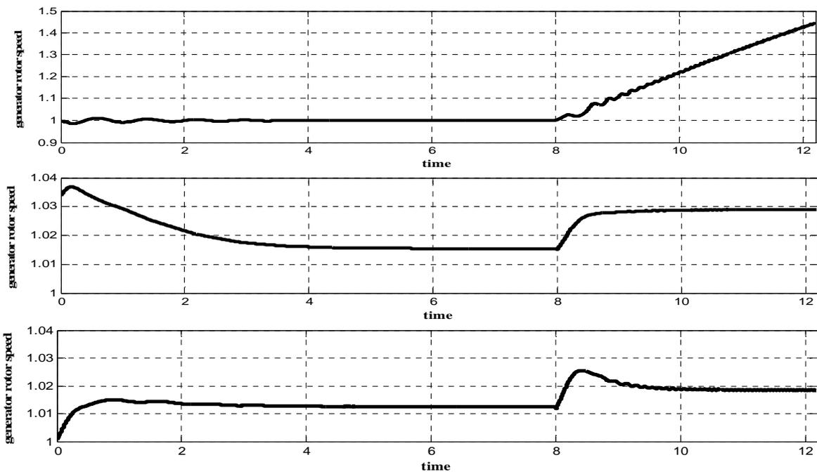
Fig.19 rotor speed of synchronous, squirrel-cage, and doubly-fed induction generators respectively pre- and after fault clearance
