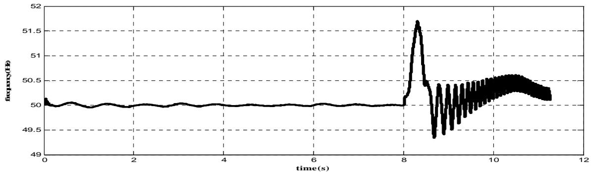
Fig.17 frequency of the power system at the point of common coupling pre- and after fault
