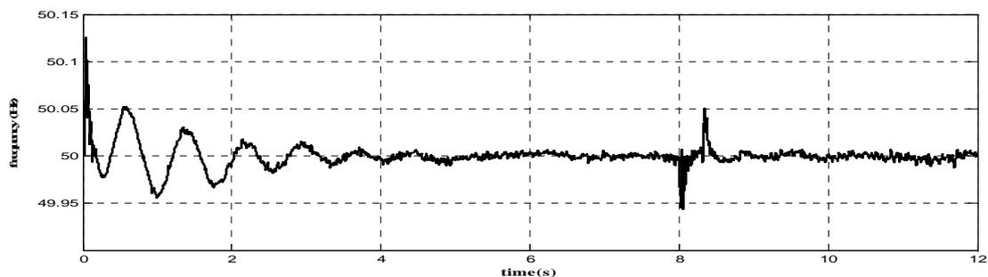
Fig. 2 Frequency of the power system at the point of common coupling pre- and after fault clearance
