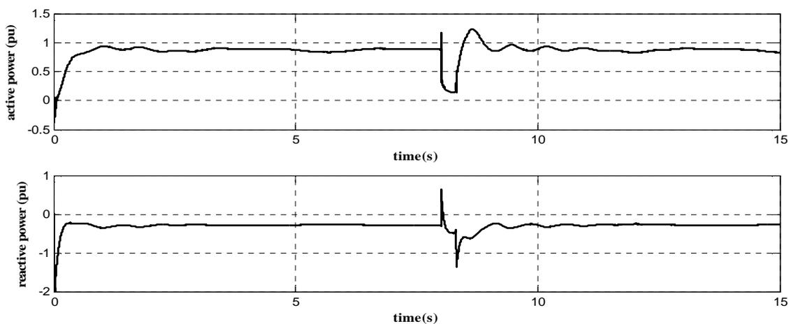
Fig.16 active and reactive power of the doubly-fed induction generator pre- and after fault clearance
