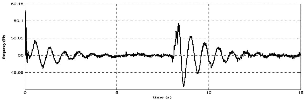
Fig.12 frequency of the power system at the point of common coupling
