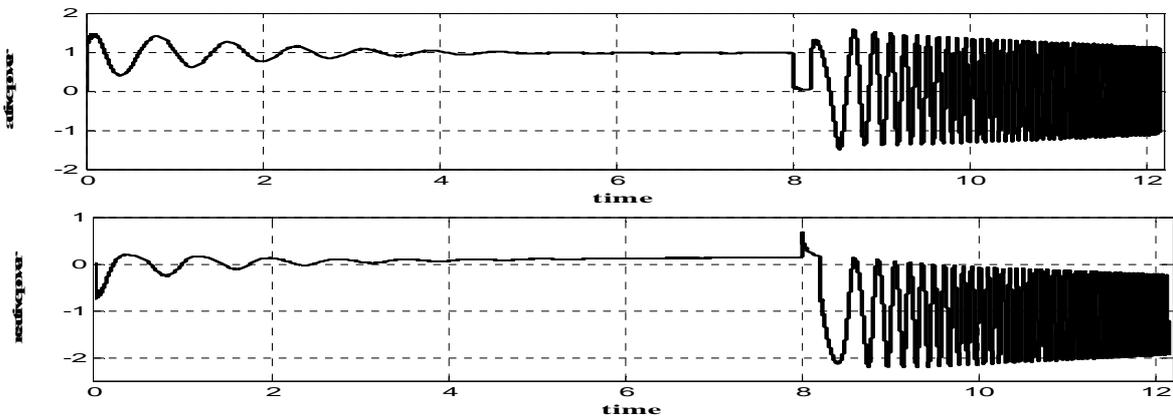
Fig. 20 active and reactive power of the synchronous generator pre- and after fault clearance
