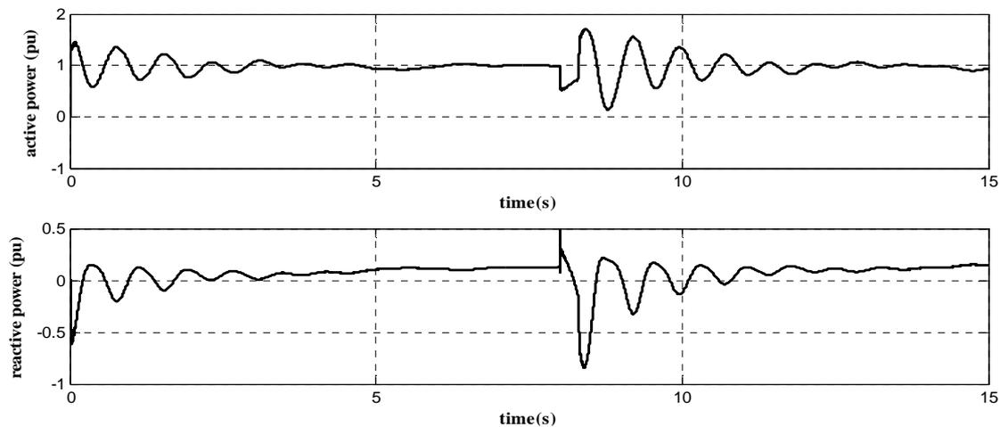
Fig.14 active and reactive power of the synchronous generator pre- and after fault clearance
