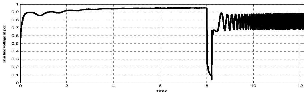
Fig.18 Rms\_voltage of the power system and at the point of common coupling pre- and after fault clearance
