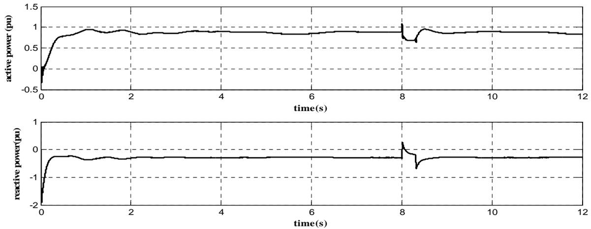
Fig.6 active and reactive power of the doubly-fed induction generator pre- and after fault clearance
