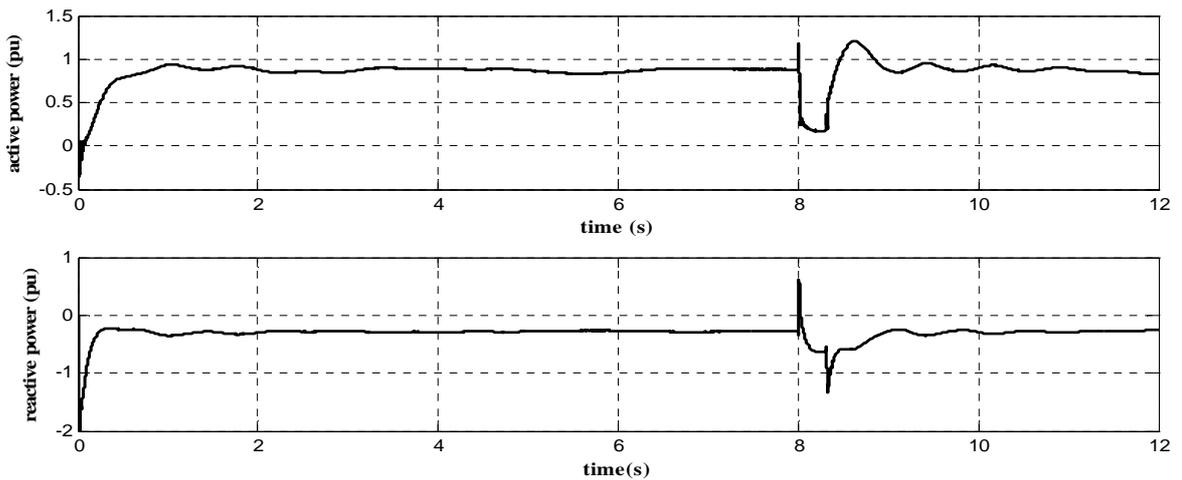
Fig. 11 active and reactive power of the doubly-fed induction generator pre- and after fault clearance
