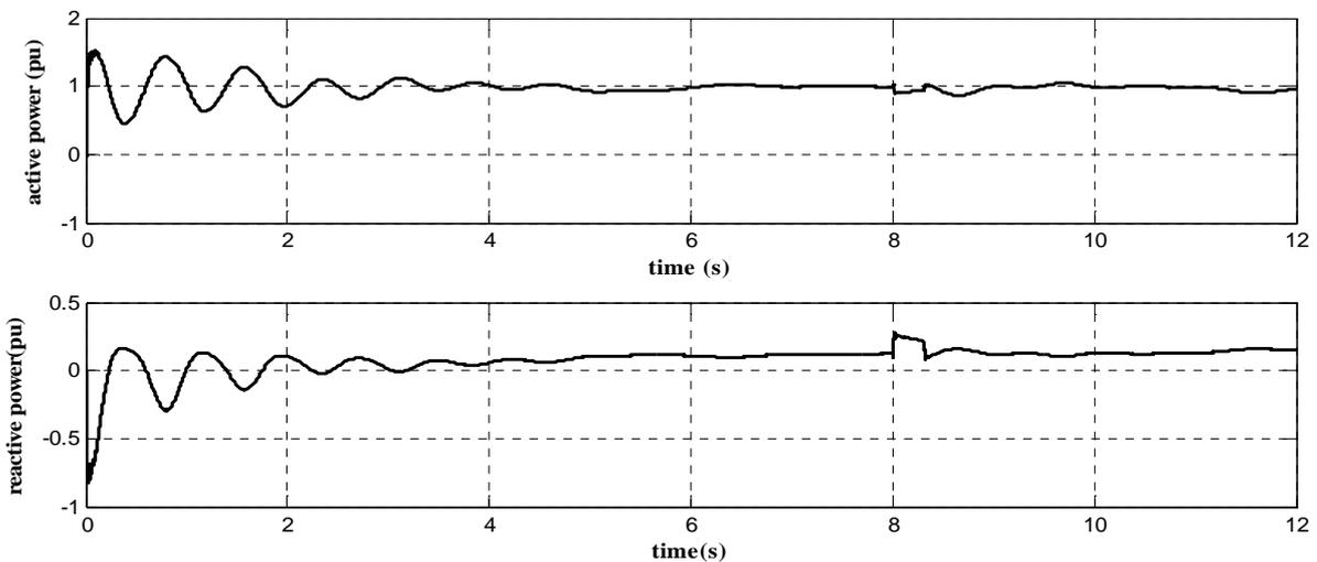
Fig.4 active and reactive power of the synchronous generator pre- and after fault clearance
