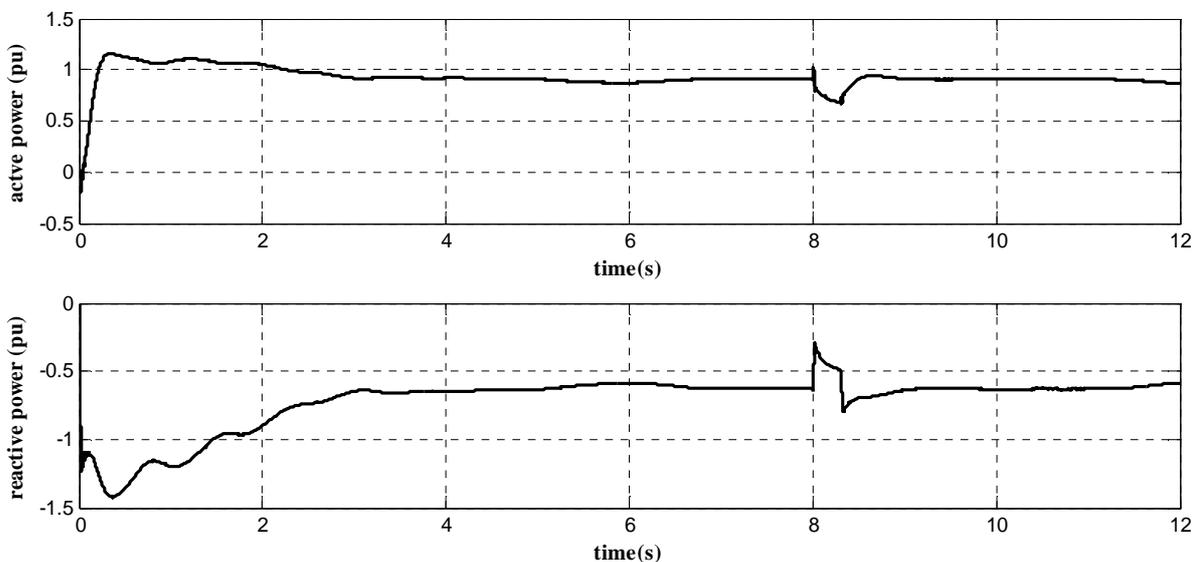
Fig.5 active and reactive power of the squirrel-cage induction generator pre- and after fault clearance
