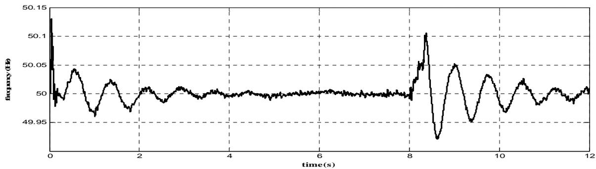
Fig. 7 frequency of the power system at the point of common
