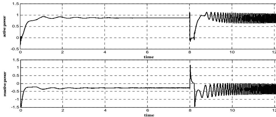
Fig.22 active and reactive power of the doubly-fed induction generator pre- and after fault clearance
