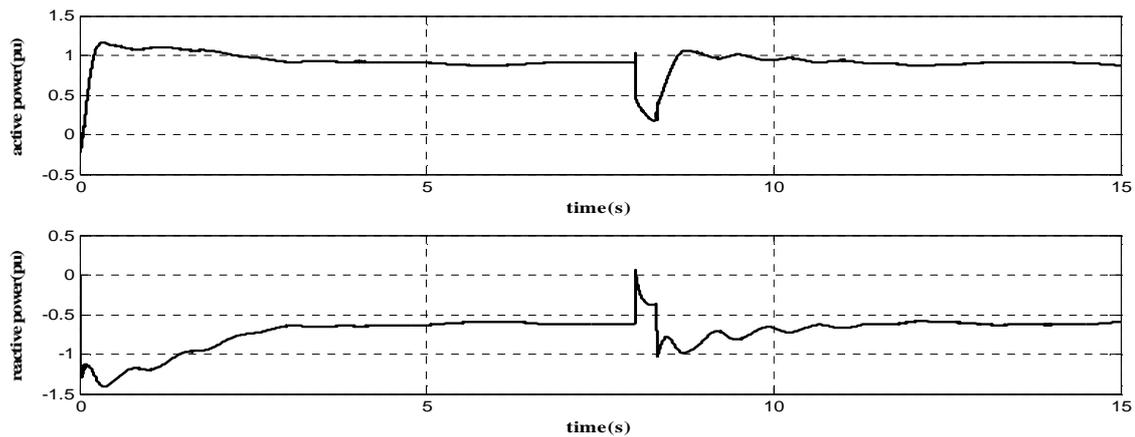
Fig.15 active and reactive power of the cage generator pre- and after fault clearance
